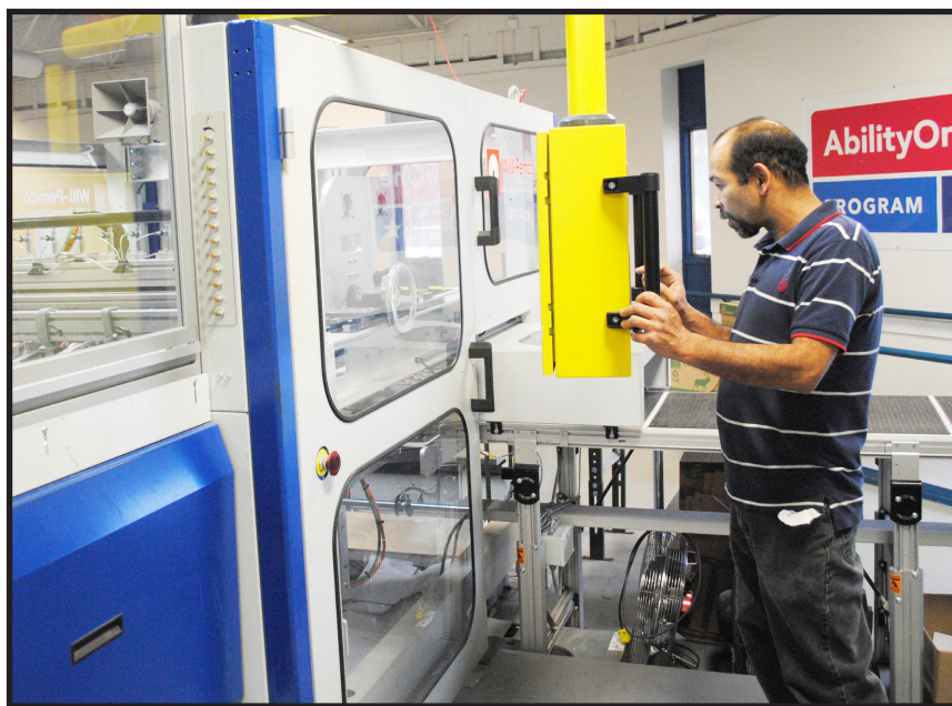
(Above) Jim alters the speed of the Will-Pemco paper sheeter to prepare for a paper roll change.
